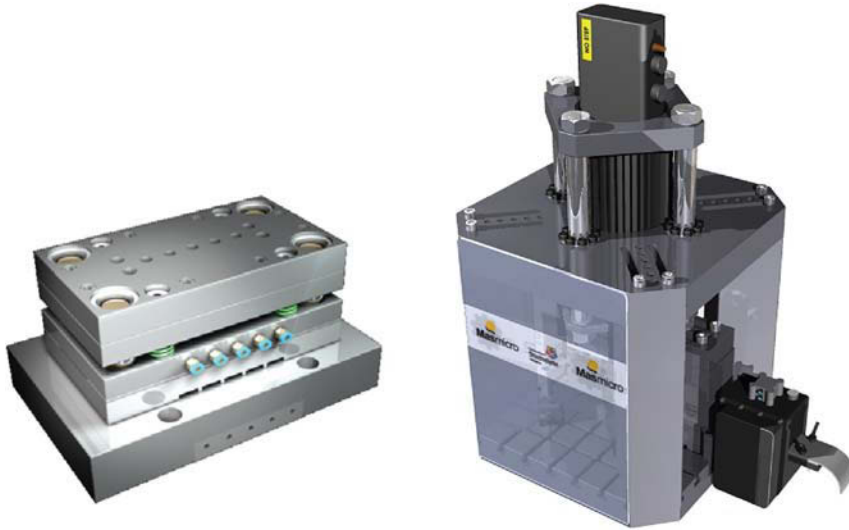
FIGURE 8-12 The micro-forming tool (left) and the micro-forming machine (right), developed at the University of Strathclyde.
