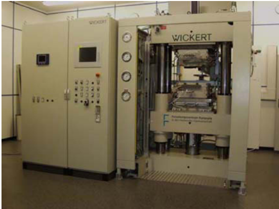
FIGURE 5-12 Hot embossing machine Wickert WMP1000.
