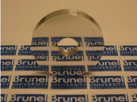
FIGURE 2-14 Mirror surface achieved on the three-axis diamond-turning machine.
