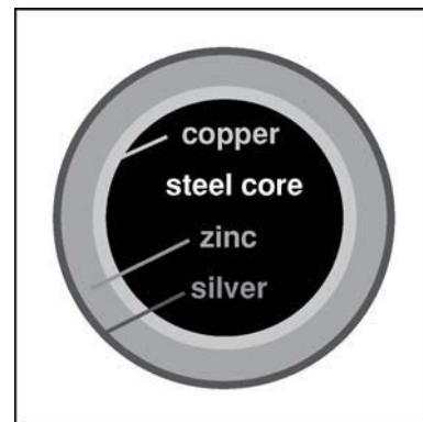
FIGURE 3-9 Build-up of a micro-multi-layer wire electrode.
