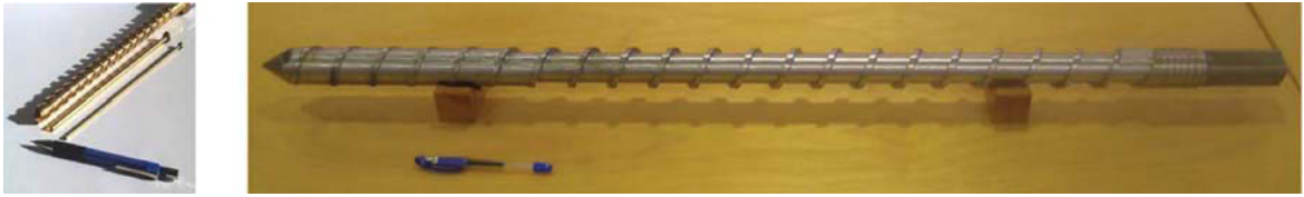
FIGURE 6-6 Comparison of dimensions between screw and injection plungers for \mu\text{M} (left) and a screw for conventional injection molding (right).
