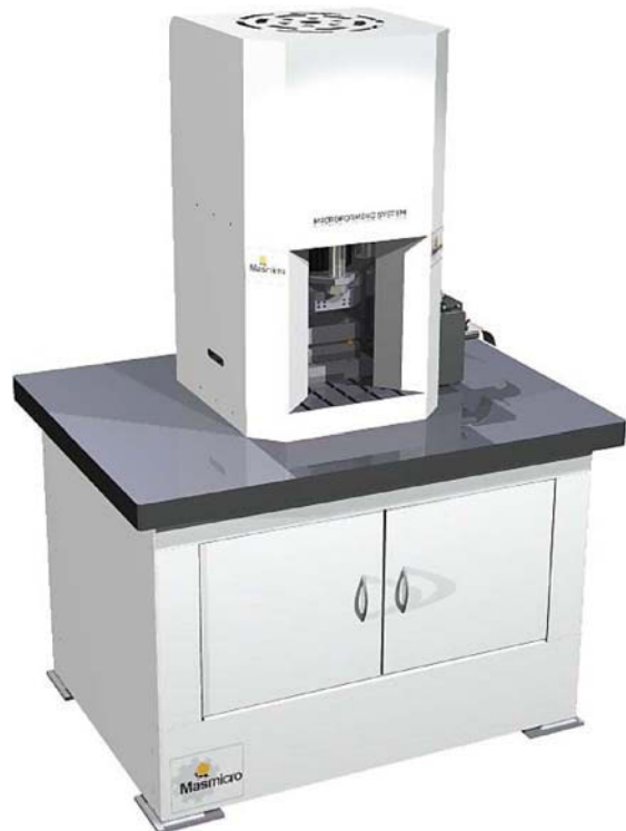
FIGURE 8-10 A bench-top micro-sheet-forming machine, designed by the University of Strathclyde.
