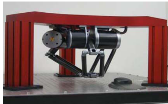
FIGURE 19-3 The Pocket Delta robot. (Source: courtesy of CSEM, SA Switzerland.)
