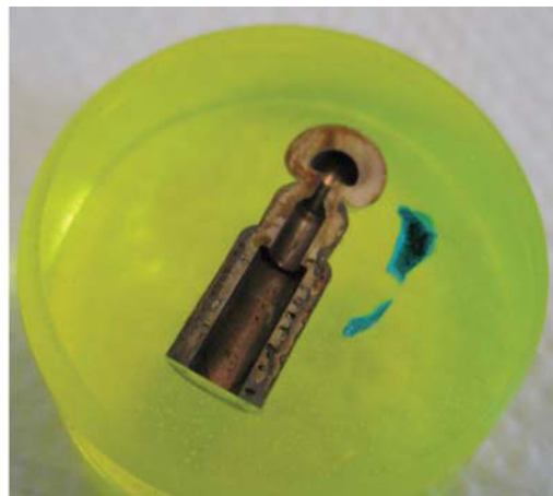
FIGURE 17-8 Indirect Approach for Dies for Micro-metal Forming. Turned Geometry (left) and Cross-section of Electroformed Die (right).
