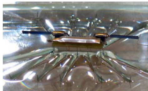
FIGURE 19-10 The Strider Micro-robot. (Source: courtesy of Metin Sitti, Nano-Robotics Laboratory, Carnegie Mellon University.)
