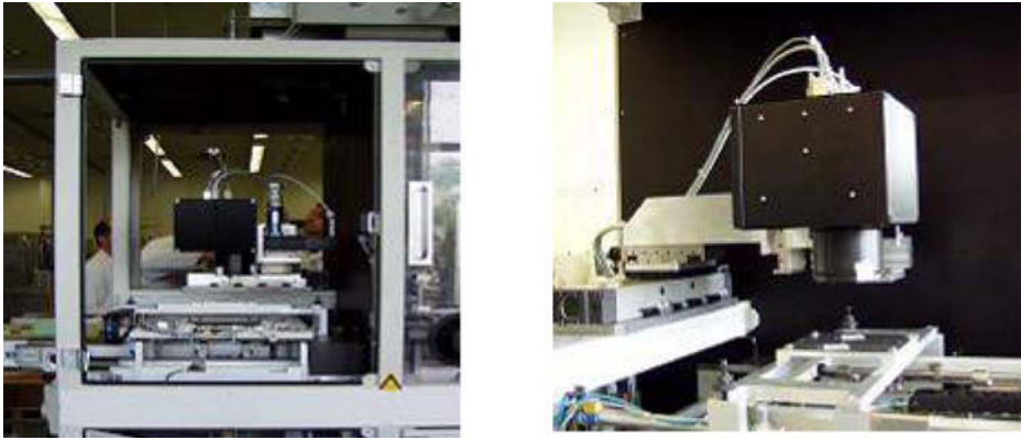
FIGURE 12-2 System design for laser beam soldering based on a galvanometric scanner: Production cell (left) and laser processing optics (right).
