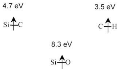
FIGURE 15-17 Bond energies of HMDSO.
