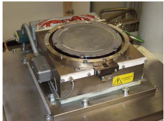
FIGURE 5-16 Lower half of a basic molding tool with a moldable surface area of up to 250 mm diameter.
